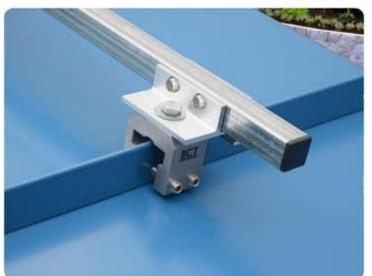
This is a 3 inch wide mounting bracket, also know as the "RCB-3 Bracket" attachment point for mounting the SnoBar and ColorBar snow rails to the standing seam RoofClamp. This bracket has a wider swivel range of 31 degrees to accommodate more severe angles on converging hips and valleys. The narrower 2 inch RCB-2 bracket only swivels 19 degrees. Bar, RoofClamp and bar mounting fasteners are NOT included.
