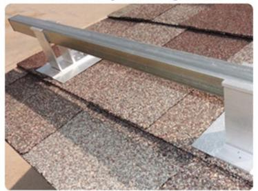
Our exclusive Shingle Mounts allow SnoBar and ColorBar products to be safely installed on shingle roof systems without causing roof leaks, shingle damage, or voided warranties. Shingle Mounts are fabricated with a 12" X 4"- 24 gauge galvalume strap, two 304 stainless steel mounting bolts, and one extruded aluminum ColorBracket mount. Four predrilled screw holes allow for mechanical fastening to new or existing roof structures.
