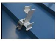
aligns with the threaded hole on top of the RoofClamp. The four smaller holes on the face of the RC-2B bracket will be facing upslope. Use the supplied top bolt and washer to attach the RC-2B bracket onto the RoofClamp using a 9/16" socket. Torque the top bolts to 90 in/lbs. This will be re-
