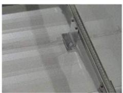
When the WINDBAR with the patented Windstopper was used on the trapezoidal panel during the ASTM E-1592 test, the flat of the roof panel was not allowed to deflect. Because it did not deflect, the seam did not fail and the ultimate failure occurred when the two(2) roof clip screws pulled out from the 16 gauge purlin.
