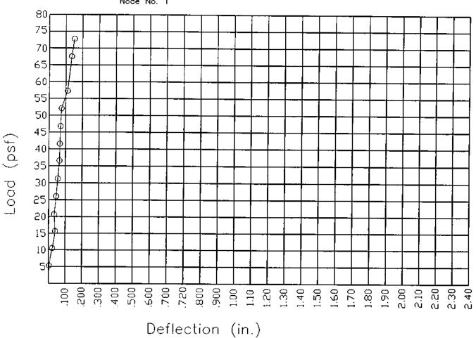
SL175 1 3/4" X 18" X 24 GA W/ WINDBAR ASTM E 1592 - Purlins @ 4'-0" Node No. 2
