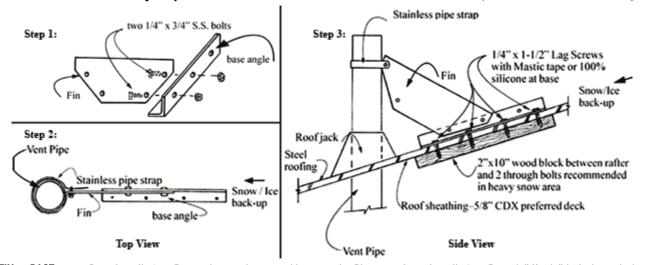
1. Attach FIN to BASE 2. Base Installation: Put sealant on bottom of base angle. Place 3. Strap Installation: Put 1/4" X 3/4" bolt through the bent end ANGLE Ventsaver centered behind pipe and fasten base to roof with the of the strap. Install as illustrated in TOP VIEW. Cut off excess Assemble with two 1/4" strap. For vent pipes cut pipe off 2" to 3" above the Ventsaver. four 1 1/2" lag screws. X 3/4" S.S. bolts. NOTE: In case of rib obstruction, base angle is reversible.
